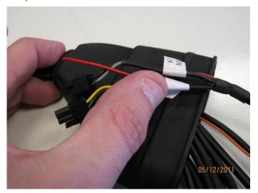
5. Insert the Battery connector through the protector hole as shown in the picture below.
