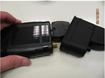
7. Cover the Cello unit with the protector part and ensure that it covers the mold tightly, as shown in the pictures below.
